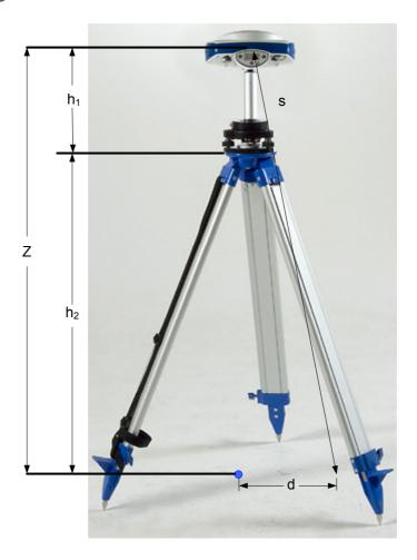
The surveyor wants height Z and is measuring slant-height s. There is an obstruction somewhere between the ProMark 500 height measurement hook and the point on the ground being measured. To calculate the error induced in the measurement s owing to the inability to measure directly to the point, one needs to know the following three values:
