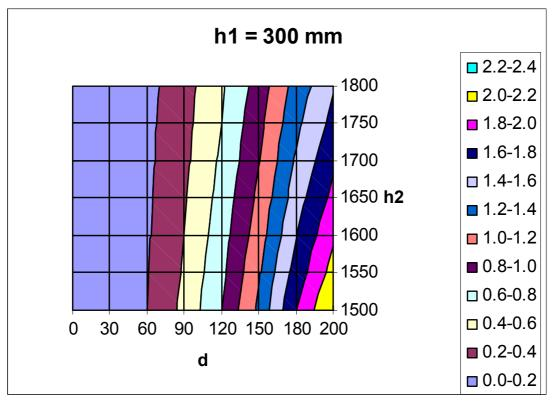
In conclusion, it is clear that the error induced by bending of the measurement tape is negligible in most situations. Care should always be taken to prevent bending the tape during slant height measurement, but small amounts of bending cause negligible error.
